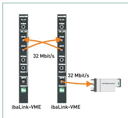
Peer-to-peer connection between two systems in the 32 Mbit/s mode with additional diagnostics
