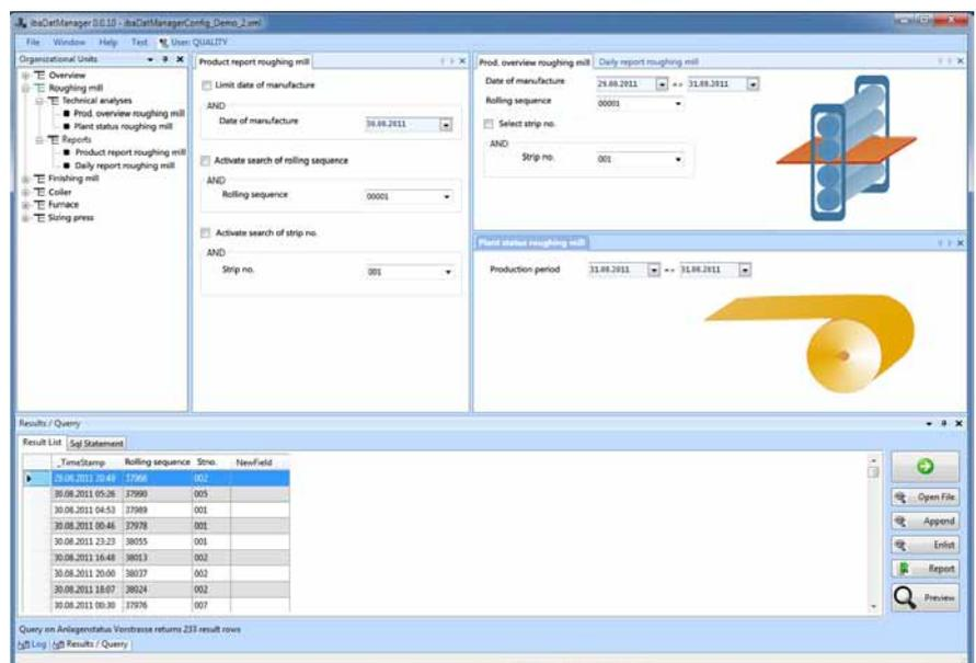
The graphic surface facilitates the search for files. Files that have been found, can be opened in ibaAnalyzer by a mouse-click.
